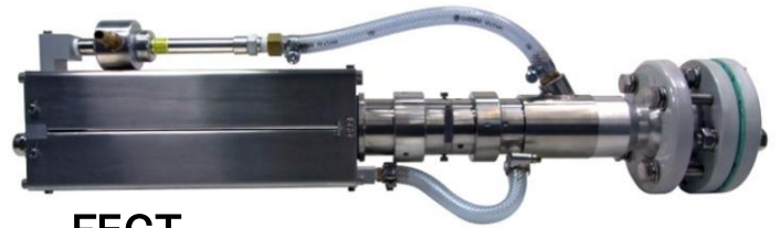
FEGT (Furnace Exit-Gas Temperature)
